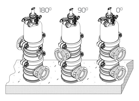
Sigma Pro 6" and 8" filters are to be installed on a flat surface only
